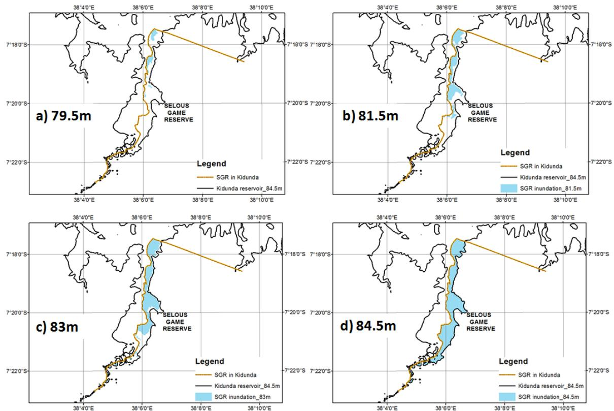
**Figure 4.8: Inundations of SGR at different reservoir elevations.**
