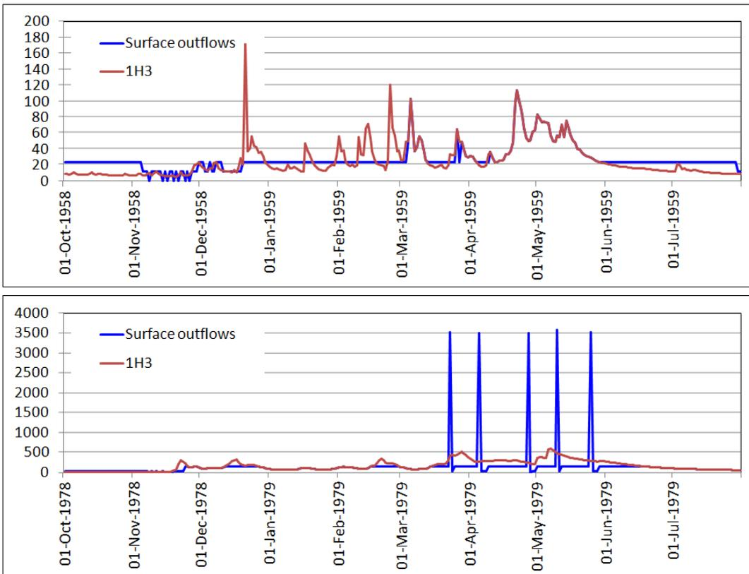
Figure 4.12: Total discharge from the dam for a fully controlled spillway (all gates closed).
