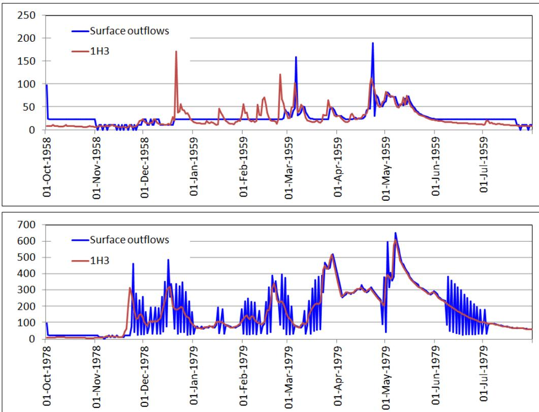
**Figure 4.9: Total discharge from the dam for an uncontrolled spillway (all gates fully open).**
