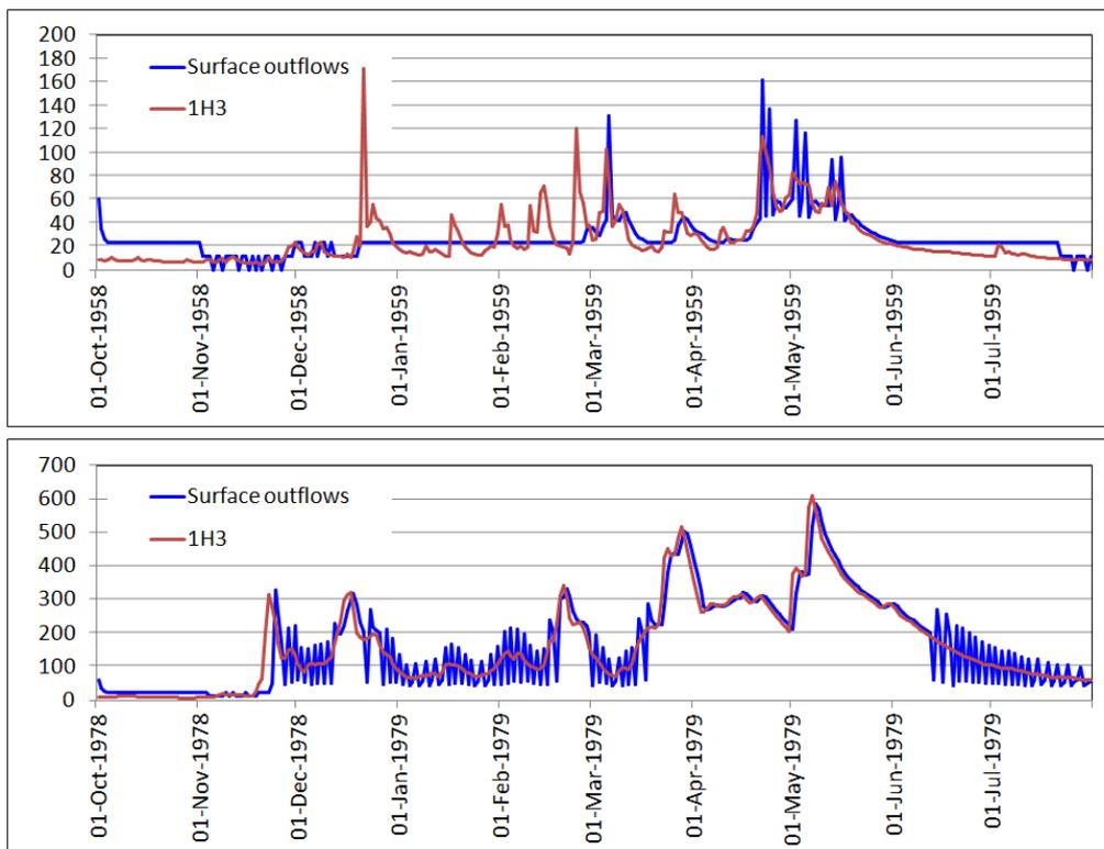
**Figure 4.10: Total discharge from the dam for a partially controlled spillway (4 gates fully open).**
