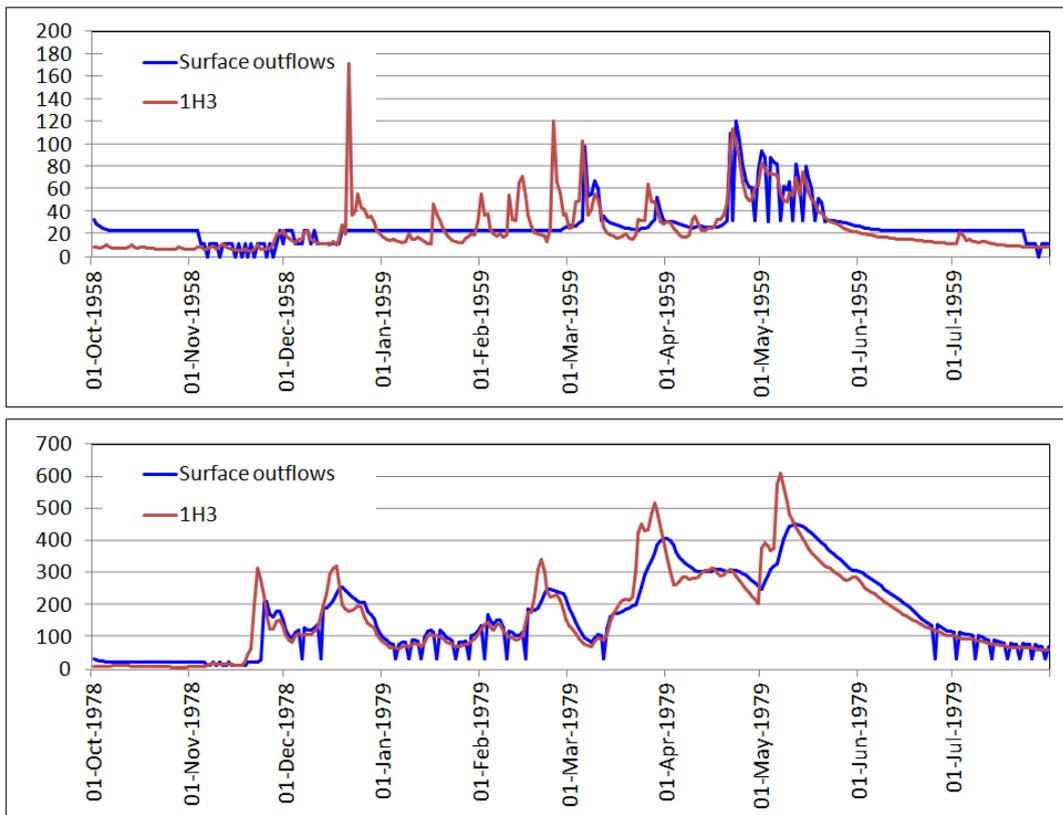
**Figure 4.11: Total discharge from the dam for a partially controlled spillway (1 gates fully open).**
